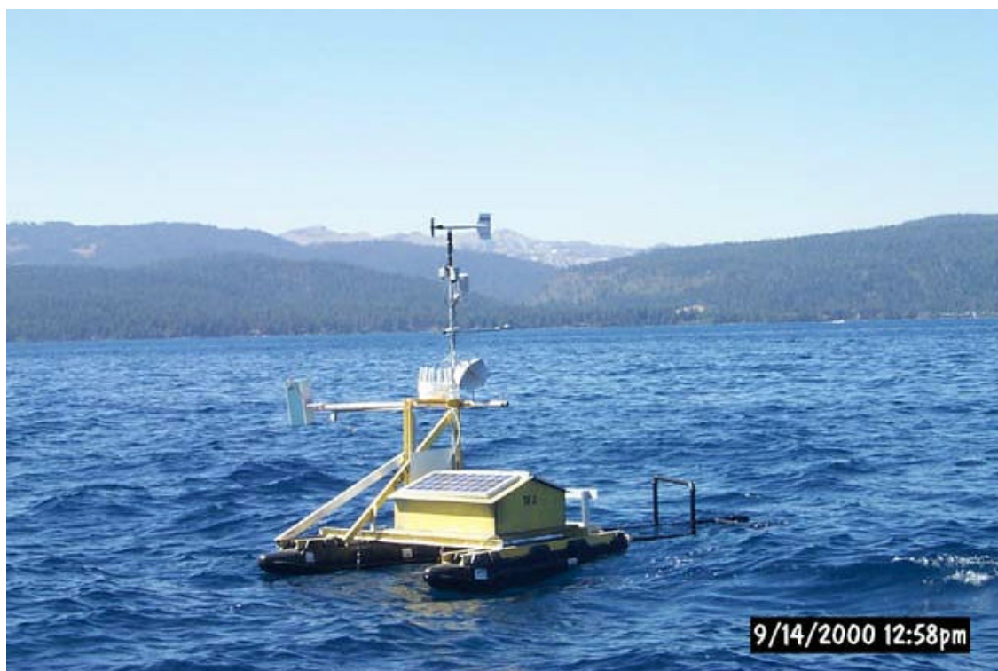
Figure 11.4.5.1-2. Surface monitoring station at TR3. The station measures the radiometric skin temperature, bulk temperature, wind direction (magnetic) and speed, relative humidity, air temperature and net radiation.
