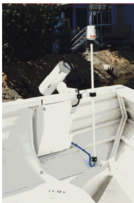
Figure 9.3.2.1-2: The Everest Radiometer fitted to the bow of a catamaran operating from Townsville to the Great Barrier Reef.
